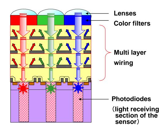
Lenses are formed on top of the sensor, with wiring between them and the light receiving section and photodiodes. Light entering the sensor obliquely is blocked by the wires, which also reflect back some to the light that enters at right angles, degrading overall light sensitivity.
