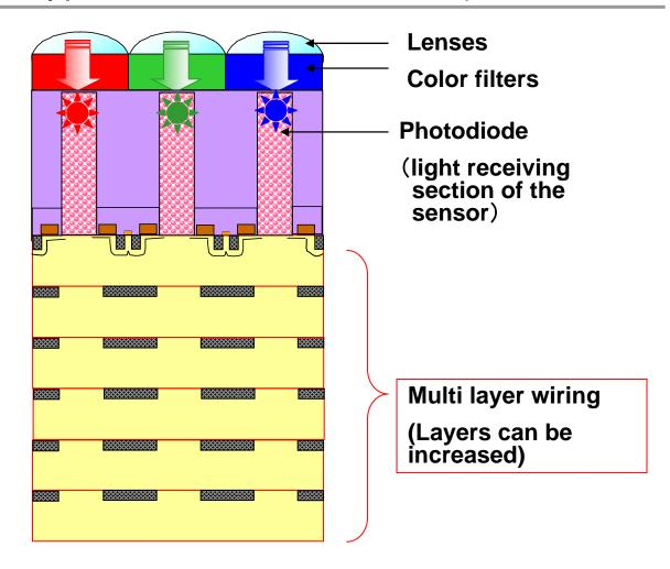
The lenses are attached to the back side of a substrate with a planed surface, and deliver light directly to the photodiodes. With no interference from wiring, light sensitivity and overall performance are boosted.
