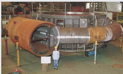
Shop assembly of pump-turbine for Kazunogawa Pumped-Storage Power Station Unit No.4 of The Tokyo Electric Power Co., Inc.
