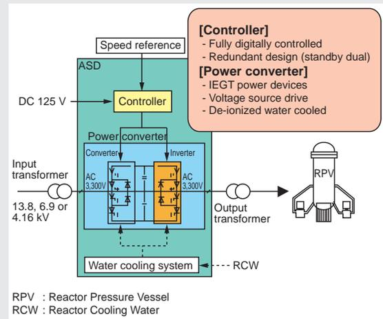
RPV : Reactor Pressure Vessel
