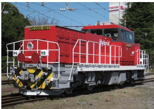
Type HD300 shunting locomotive with diesel hybrid system
