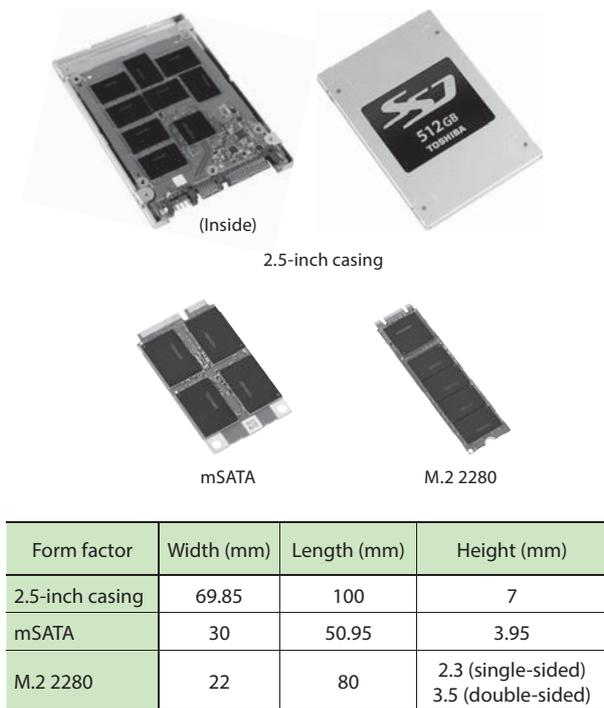
**Figure 1. Trends in reduction of form factor of client SSDs.**
