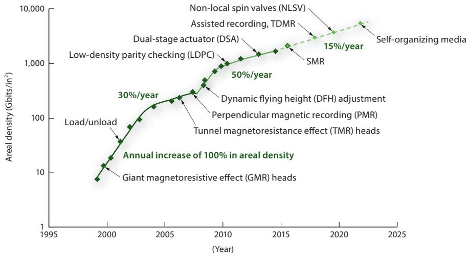
**Figure 8. Trends in areal density of HDDs and innovation technologies.**
