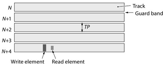
**Figure 3. Schematic diagram of data tracks, write element, and read element of high tracks per inch (TPI) CMR HDD.**
