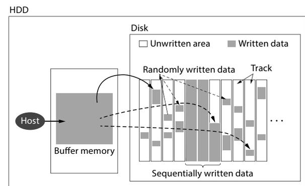
**Figure 5. Data writing procedure in CMR HDD.**
