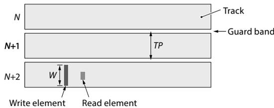
**Figure 2. Schematic diagram of data tracks, write element, and read element of conventional magnetic recording (CMR) HDD.**
