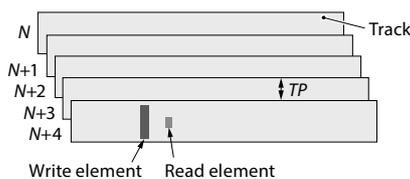
**Figure 4. Schematic diagram of data tracks, write element, and read element of high-TPI SMR HDD.**
