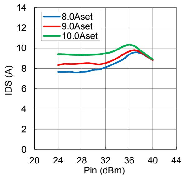
**·Pout , Gain , PAE , IDS vs. Pin vs. Temperature**
