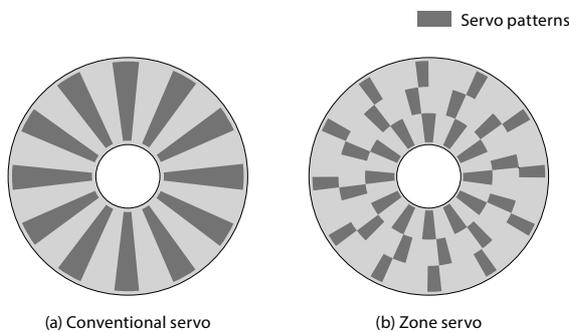
**Figure 8. Comparison of servo patterns of conventional and zoned servos.**
