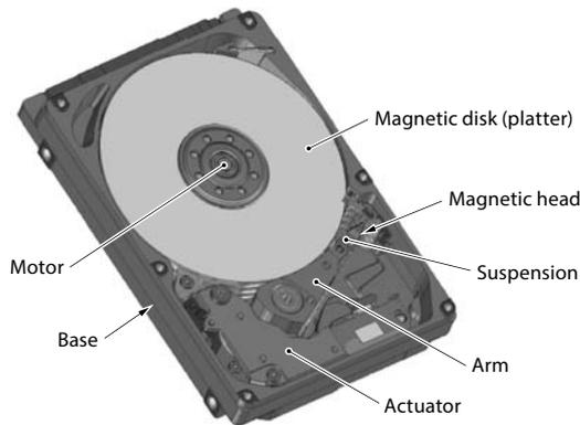
**Figure 1. Internal structure of MQ03ABB300.**
