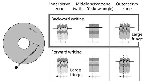
**Figure 9. Differences in side fringe according to direction of servo pattern writing.**
