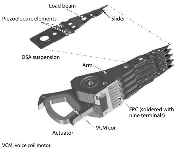
**Figure 2. Newly developed actuator and DSA suspension.**
