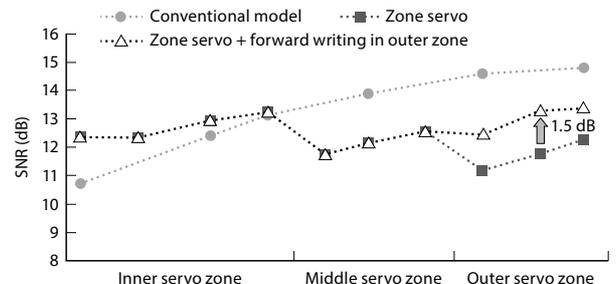
**Figure 10. Improvement of SNR of servo pattern by forward writing at outer servo zones.**
