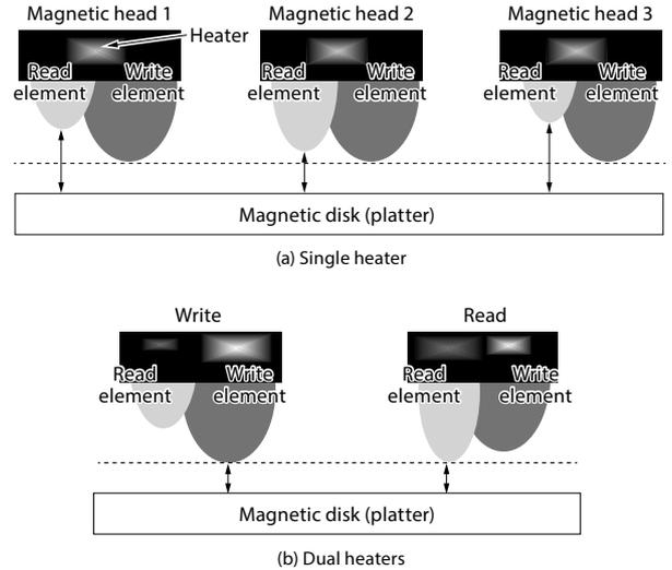
**Figure 5. Comparison of protrusion shapes of write and read elements with single and dual heaters.**
